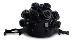
Inspired by our Flow2 system, the 12-module DevKit offers a more flexible and adaptable approach to neuroscience experimentation and data collection. By employing a soft cap design that allows users to customize and install optical modules and EEG electrodes as desired, researchers can optimize sensor placement for their specific research goals.
